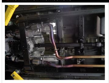
Step 1: To remove the OEM system first unbolt both inlet pipes at the catalytic converter flange junctions. Working front to rear disengage all welded hangers from the rubber insulators. The OEM exhaust system can now be removed in one piece. Be sure to retain all mounting hardware as it will be needed to install your new MAGNAFLOW system
