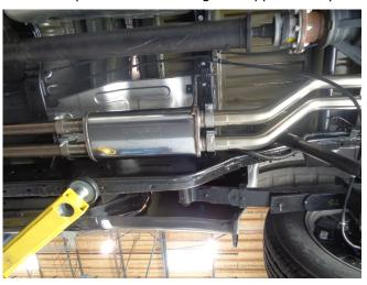
Step 4: Loosely attach the Muffler Assembly to the Extension Pipes using the supplied 2.25" clamps and engaging the welded hanger into the rubber insulator. Next install the Over Axle Pipes to the outlets of the Muffler Assembly using the supplied 2.50" clamps. (These pipes are identical).
