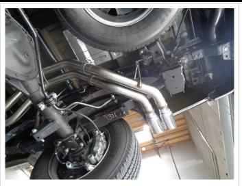
Step 5: Finish by installing the Tailpipe Assembly to the Over Axle pipes using the supplied 2.50" clamps and fitting the hanger into the rubber insulator.
