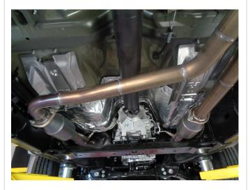
Step 2: Begin installing your new system by loosely bolting both inlet flanges of the D/S and P/S Inlet Pipe Assemblies to the catalytic converter outlets using the OEM hardware. Engage the D/S hanger to the rubber insulator.
